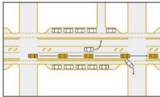
In a 3-lane configuration, the weaving and conflicts are eliminated.
